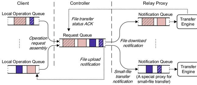
Fig. 11. The complete filesystem operation control process of HyCloud (operation requests from different clients are scheduled in the controller).
